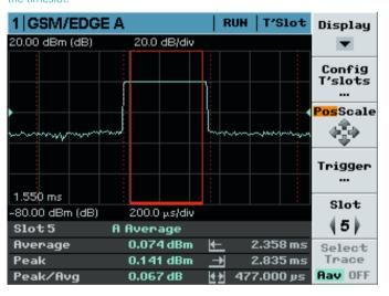
Numerical display of two continuous average measurements and their relation.
