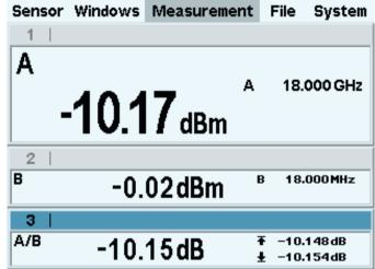
Determination of the power of an EDGE burst with the R&S®NRP-Z81 wideband power sensor using the gate function; exclusion of the training sequence in the center of the signal.
